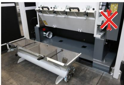
Access without tools to the main parts subject to ordinary maintenance. Maintenance from one side only without tilting.
