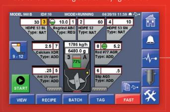
**FlexBus Lite** is integrated with our touchscreen controller for loading multiple materials into a blender.
