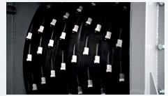
The ZRS uses very large diameter flat E-style rotors. Knives are fixed in special knife holders fitted in machined pockets.
