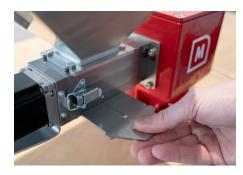
**Easy drainage**Discharge valve for quick draining of hopper and dosing house contents.
