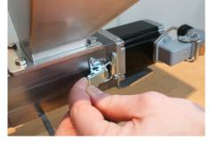
**Simple motor removal**Open the two latches to release the motor and easily clean the dosing house.
