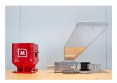
**Convenient maintenance** Feeder can be positioned upright for convenient maintenance, cleaning and calibration.
