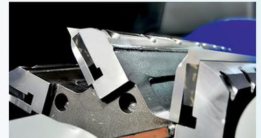
For abrasive applications GSH granulators can be equipped with rotors with key parts manufactured from highly wear resistant steel as well as weld on hard facing.
