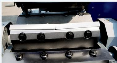
GSH granulators are available with different rotor options to fit different applications, all rotors feature the V-cut technology creating a high quality regrind.
