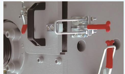
The Quick Snap System allows the lower front plate section to be easily removed for granulator cleaning. The lower front plate section is held in position by two sturdy lever clamps.
