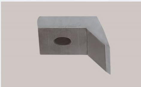
The curvature of the specially profiled rotor knives ensures a constant cutting radius after re-sharpening thus maintaining the original cutting gap. Awkward knife adjustment is no longer necessary.
