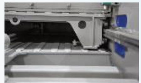
The ZCS system uses a sturdy roller guided drawer type ram to feed the material into the shredder. Segmented cutting chamber and ram allow trouble free processing of thin materials.
