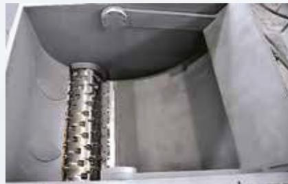
The internal ram design on the ZIS series allows the cutting chamber volume to be increased while keeping a small footprint. Making the ZIS ideal for shredding of big volume parts.
