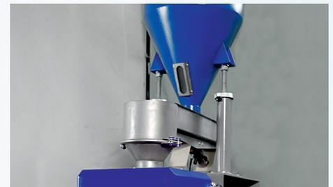
Material is fed into the pulverizer by a vibrating dosing channel, the feeding rate is automatically adjusted based on the motors amperage and material temperature.
