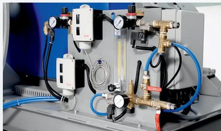
Material temperature is monitored in the process. An automated cooling system ensures temperature is kept at a defined level.
