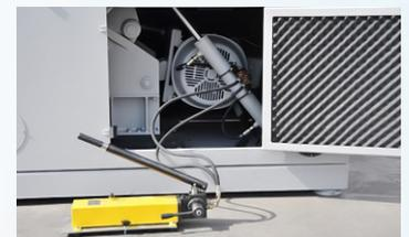
The GSC 500 machine's cutting chamber is opened hydraulically for safety
