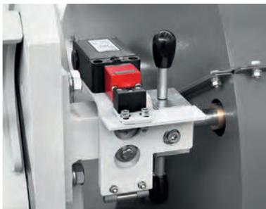
Rotor lock for maintenance. Safety devices and circuit in compliance with EEC Directives.
