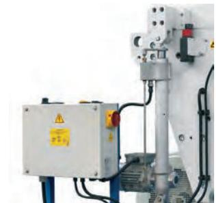
Hopper opening with motorized jack and screen-holder opening by gas cylinder.
