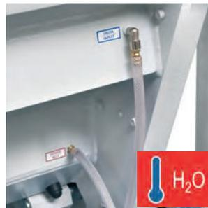
Chamber water cooling. Screen equal to approximately 50% of blades rotation length.
